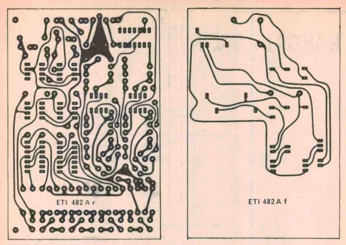
Fig 7. Printed circuit layout(both sides) of the preamp board. Full size 120 x 80 mm.
