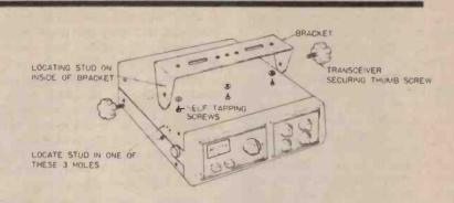
Fig. 1. Typical Transceiver Mounting.
