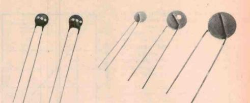
Fig. 10. Typical PTC thermistors (actual size).
