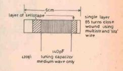
Fig. 2. Coil winding details
