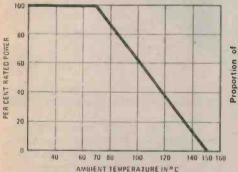
Proportion of Rated Dissipation % POWER RATED 50 64 50 PEACENT 36 0 40 60 80 100 120 140 155 Ambient Temperature °C
