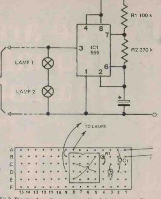
Fig.3. The view from the non-copper side of the Veroboard. The two link wires shown under the IC are not on the top of the board – they should be made on the copper side.
