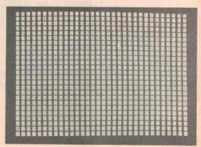
Test pattern with the ROM removed.
