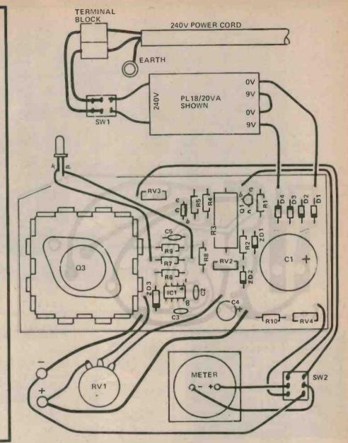
Fig 3. The component overlay and interconection diagram.
