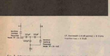
Fig. 7. Alternative resonator system giving better noise figures.
