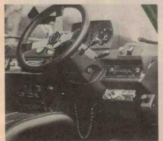
Fig. 2. This photo shows a 23-channel transceiver mounted in a Range-Rover. Note the loudspeaker is mounted on the bottom of the case which is OK when the unit is mounted under the dash but would be unsatisfactory if it had been mounted in the dash itself (like the radio in this picture). In this case an extension loudspeaker should be used.
