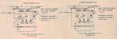
Fig. 5. Suppressing regulator noise - typical methods.
