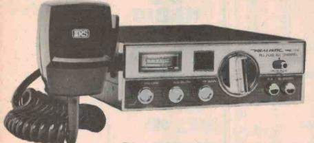
This new transceiver is shortly to be available from Tandy stores. It gives LED readout of the channel number and features a PLL synthesiser (you don't have to buy extra crystals to get all channels).
