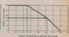
Fig. 1. Derating curve for most common metal F blaze resistors - common to the majority of film resistors.
