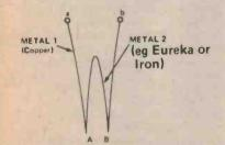
perature difference exists between the junction a and b. This voltage varies almost linearly with temperature for differences up to about 100°C, although this assumption should not be made in calibrating the thermometer for accurate measurement.
