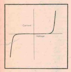
Fig 12. Varistor voltage-current characteristics.
