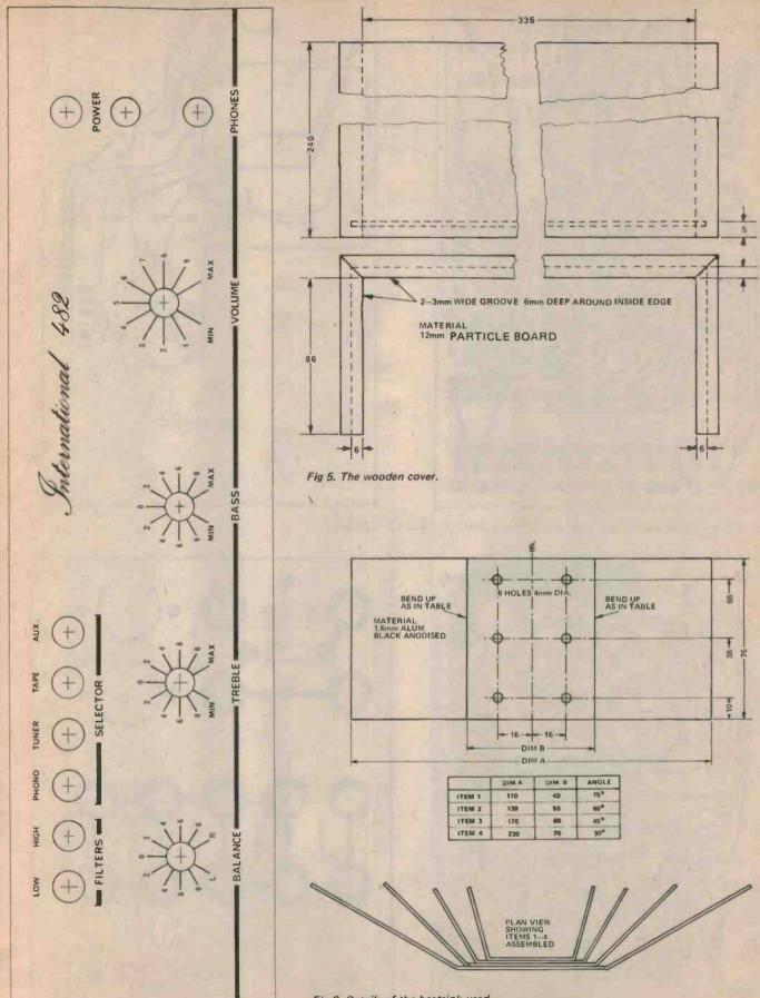
Fig 6. Details of the heatsink used.
