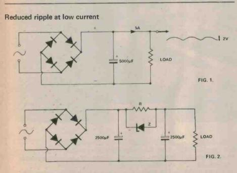
In the normal circuit (Fig. 1) the ripple at 1 amp is at least 2 volts. Cheap power amps use this circuit (with low supply ripple rejection) and produce annoying amounts of hum at low signal levels.
