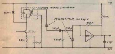
Fig. 9. Alternative resonator circuit.
