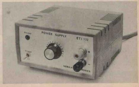
The photo on the right shows the second version of the power supply — where the voltage is set using a calibrated pot rather than a meter.
