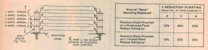
Fig. 8. Recommended method of stacking the flat style of wirewound resistors and the necessary power derating. No more than four resistors should be in a stack,
