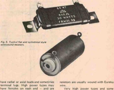
Very high power types and some very low resistance types are sometimes wound with flat-tape element instead of wire. It is usually wound edge-on to the bobbin to improve heat dissipation from the element.
