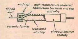
Fig. 4. Typical construction of small, cylindrical style wirewound resistor.
