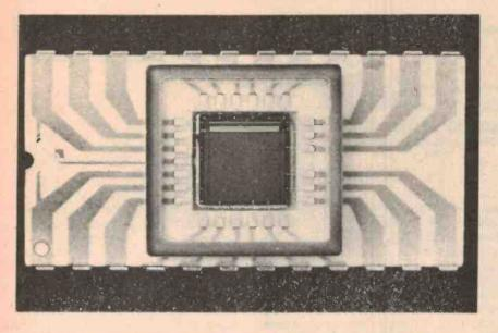
Fig. 3. Solid-state sensing array research is paving the way to tricolour LED panel televisions of the future. This unit has  $64 \times 64$  photo diodes integrated into 6 mm square.
