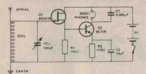
The circuit shown in the figure provides a simple radio receiver which is both sensitive and selective. A lowcost FET is used – the JUGFET 2N3819.
