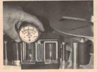
**Check Magnetism in Recorder Components** The Annis Pocket Magnetometer quickly and accurately measures residual magnetism levels in recorder heads, drive capstans or tape guides. Indicates when it's time to demagnetize and lets you know when it's again safe to use the recorder.
