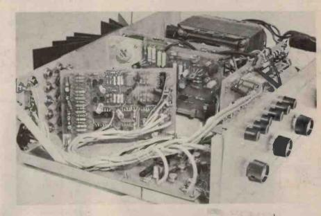
An internal view of the amplifier. Note that the preamp baord is pivoted out and not in its final position which is parallel with the rear of the unit.
