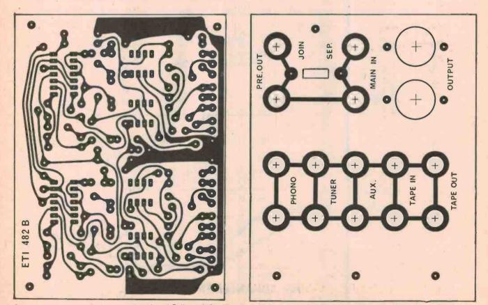
Fig 8. Printed circuit layout of the tone control board. Full size 110 x 80 mm. Fig 9. Details of the rear panel. Material 1.6mm fibreglass 1oz cu board.
