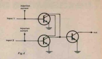
the isolated collector outputs as shown in Fig. 4. Similarly NAND gates can be made by using the multiple collector outputs of the npn transistor connected as shown in Fig. 5.
